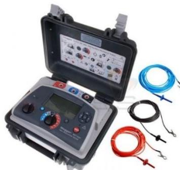
Figure 6-2 Megger Insulation Resistance Tester
