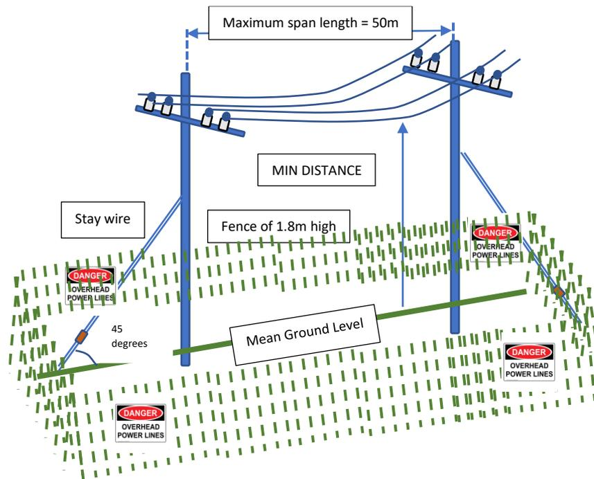
**Figure 5-3 Sketch of the front view on MAD and Clearance Distance**
