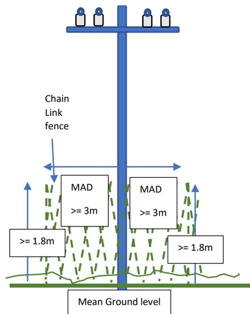
**Figure 5-2 Sketch of the side view of MAD and Clearance**
