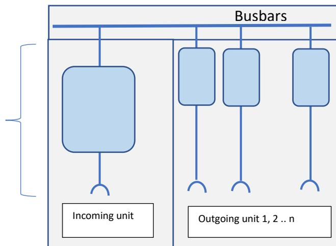
**Figure 6-1 Internal Separation**
