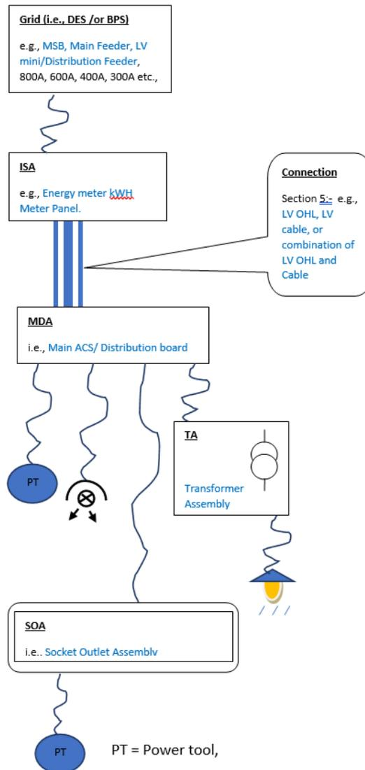
**Figure 5-1 Typical Block Diagram of Voltage Selection**
